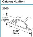
Base and Cover – Cover: .050" [1.25mm] galvanized steel. Base: .040" [1mm] galvanized steel. Packed (5) 10 ft. [3.050m] lengths per carton. Base has 9/32" [7.1mm] dia. mounting holes on centers of approximately 8" [203mm].
