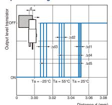
$\label{eq:continuous} Distance~d~(mm)$  Vcc =12 V, No. of repetitions: 20,  $\Delta d1=0.002~mm,~\Delta d2=0.004~mm,~\Delta d3=0.005~mm,~\Delta d4=0.02~mm,~\Delta d5=0.04~mm$
