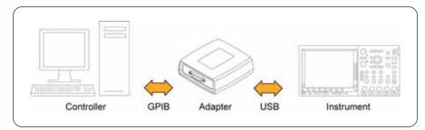
► Adapter configuration to controller and instrument.
