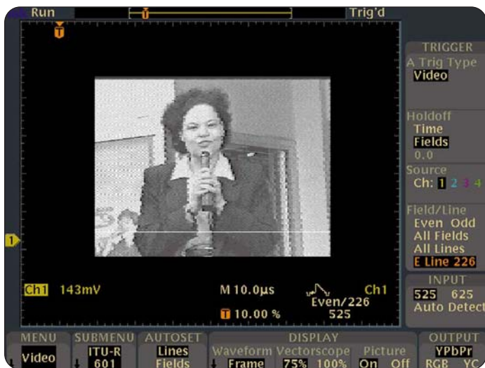
▶ Figure 2. The optional video module lets you see the signal as monochrome display with on-screen line select.
