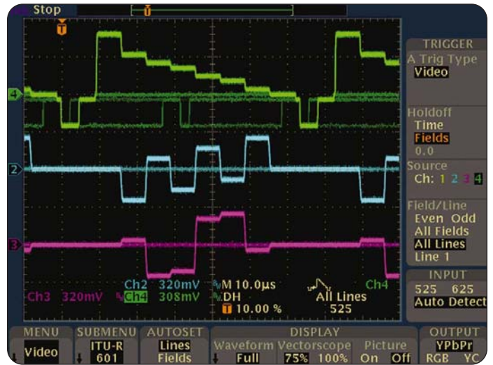
► Figure 7. TDS3SDI decoding of the 601 bit stream showing Y_p P_r .
