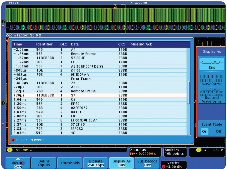
► Packet decode table showing decoded Identifier, DLC, Data and CRC for every CAN packet in a long acquisition.
