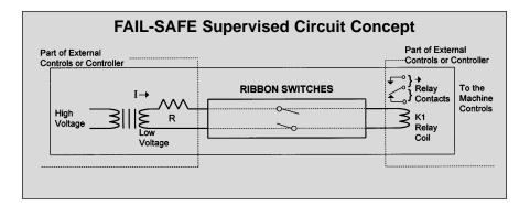
or critical alarm circuits. See Interface Controllers Section for a detailed explanation of the concept. The functional safety of the Tapeswitch fulfills Class 2.2 (category 3 prEN954-1) when used with a suitable, control reliable controller, (such as the PSSU Series).
