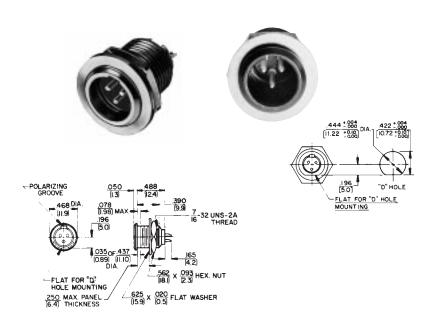
Male receptacle for chassis/panel mounting. Specially designed flange permits close (front) mount on crowded panels. Mounting hardware supplied.
