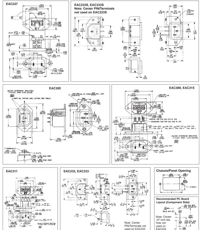
Note: Unless otherwise specified, all dimension tolerances are  $\pm$  .01 inch (+0.25 mm)
