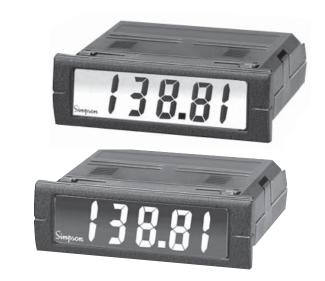
Simpson's Mini-Max Current Indicators provide high quality, accuracy and reliability in a compact, 60mm deep case. Units offer 4-1/2 digit, 0.5" (12.7mm) LCD display and are available with a bright red, negative image backlight option. All units feature user-selectable decimal point, auto zero and limited scaling capabilities.
