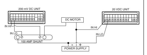
lead of the shunt is connected to the IN HI terminal, and the negative lead connected to the IN LO terminal. The Mini-Max units will indicate the power supply voltage and load current of the motor.
