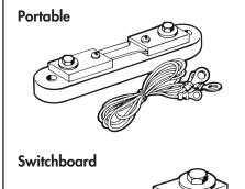
External shunts enable digital panel meters to indicate higher currents than can be provided with self-contained internal shunt meters. The shunt is installed in series with the load and source. The shunts produce a DCmV drop which is sent to the display unit. The Mini-Max can be scaled to display the actual current between the load and the source. Simpson manufactures portable and switchboard shunts.
