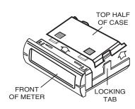
Using a screwdriver or thumbnail, spread tab on each side of case to unlock top half. Lift rear top half and slide away from front of meter.
