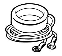
Donut Current Transformers enable the Mini-Max to monitor AC current up to 1999 amps. The Donut (also known as a "Toroid") is placed around one of the legs of the device being monitored, and emits up to a 5 amp signal. The Mini-Max can be scaled to accurately display the current being monitored. Each Donut comes with 2' long secondary leads.
