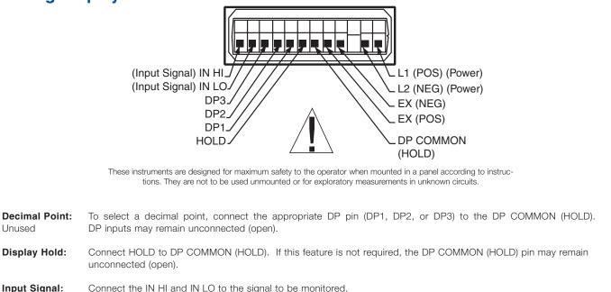
Input Power: Connect power to the L1 and L2 terminals. For AC powered units, L1 and L2 are not polarized. For 9-32 DC powered units, L1 must be positive with respect to L2.
