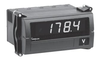
Compactly designed for applications requiring minimal rear panel depth, the Falcon fits a standard 1/8 DIN panel cutout (91.9mm x 45mm) and requires less than 3" behind the panel. A screw terminal connector is a standard feature for easy wiring of the power supply and signal input connections
