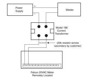
The current transformer is installed in series between the power supply and the welding process. The Falcon AC volt meter is connected to the transformer.
