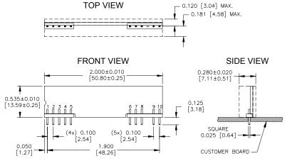
YNV05T16 Pinout (Through Hole - SIP)
