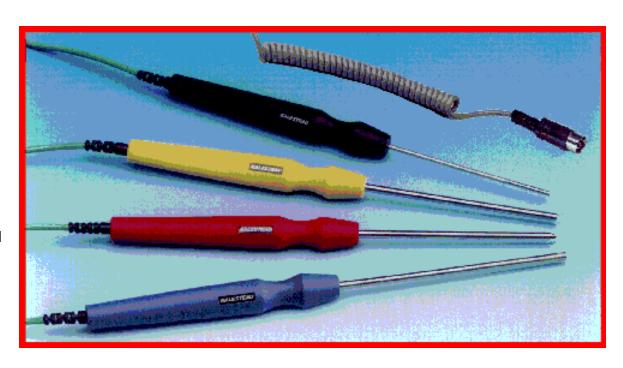
Pico Technology supplies a range of Class A sensors ( $\pm 0.15$  at 0 °C) and tenth-DIN sensors ( $\pm 0.03$  at 0 °C). Specialist manufacturers can provide sensors with 0.001 at 0 °C accuracy (at a price). Please note that these accuracy specifications relate to the SENSOR ONLY. It is necessary to add the sensor error to the PT-104 error.
