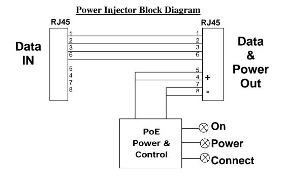
**Description of LED Functions for Power Injector**
