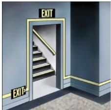
• Used to mark egress routes, fire alarms, and fire equipment that is clearly visible for up to ten hours after power is lost
