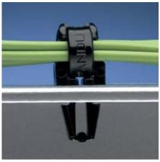
• Push mounts require no adhesive backing or additional mounting hardware. They are inserted into pre-drilled holes. Can be used where only one side of the panel is accessible. This push mount does not have tensioning wings.
