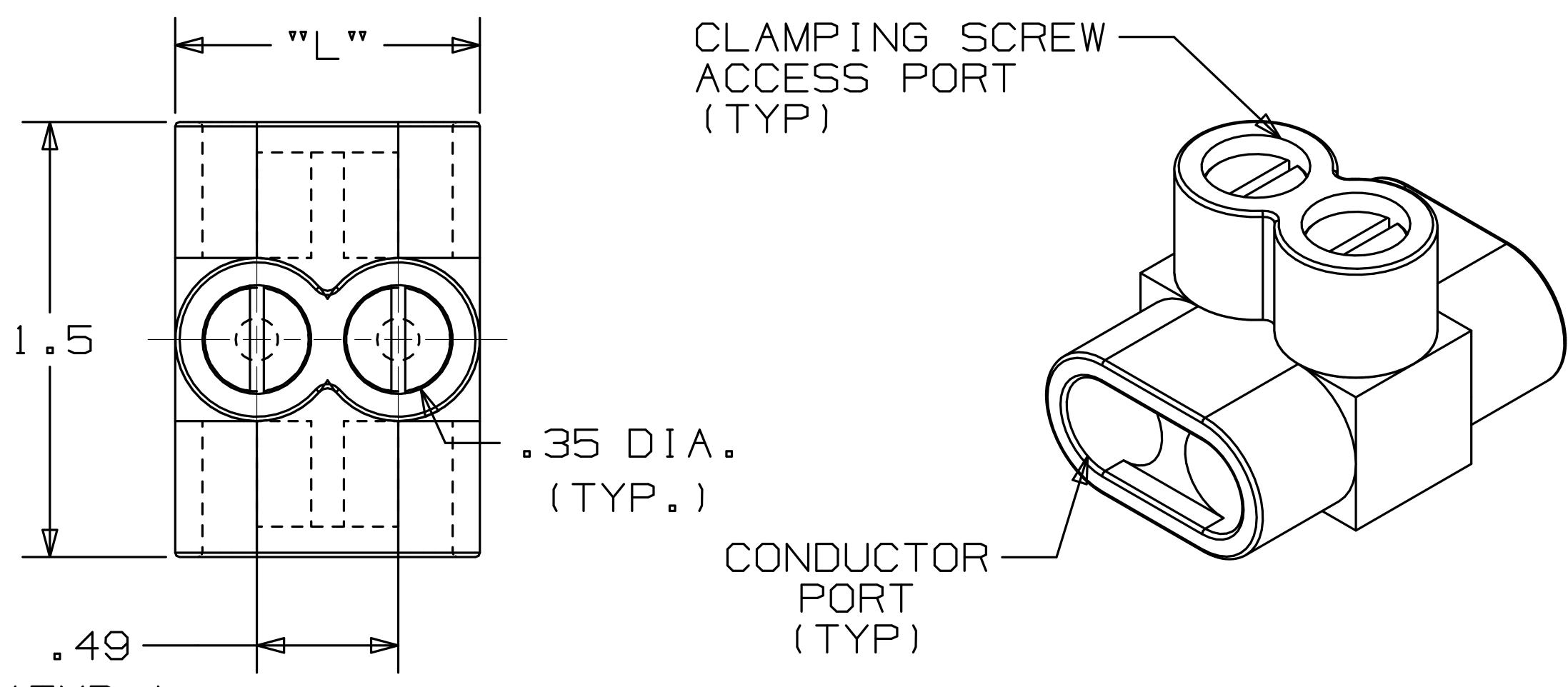
TWO PORT CONNECTOR BLOCK SHOWN WITH PLASTIC CLOSURE PLUGS REMOVED. SEE TABLE FOR DIMENSIONS OF PARTS WITH ADDITIONAL PORTS.
