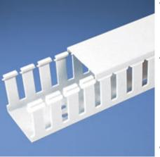
• Choose from 36 sizes of *PANDUIT®* Type G Wiring Duct from 0.5 "x 0.5" up to 6" x 4" in popular colors. Used for general purpose control panel wiring and to route and protect wiring in communication closets. The non-slip cover conceals all wiring and is easy to install. The duct and cover form a flush sidewall providing increased capacity and improved aesthetics.
