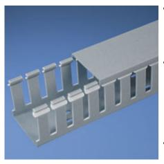
• Choose from 36 sizes of *PANDUIT®* Type G Wiring Duct from 0.5 "x 0.5" up to 6.0" x 4.0" in popular colors. Used for general purpose control panel wiring and to route and protect wiring in communication closets. The non-slip cover conceals all wiring and is easy to install. The duct and cover form a flush sidewall providing increased capacity and improved aesthetics.
