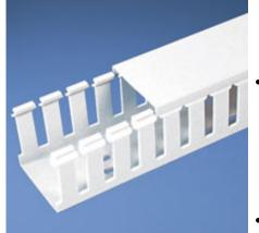
• Choose from 36 sizes of *PANDUIT®* Type G Wiring Duct from 0.5 "x 0.5" up to 6" x 4" in popular colors. Used for general purpose control panel wiring and to route and protect wiring in communication closets. The non-slip cover conceals all wiring and is easy to install. The duct and cover form a flush sidewall providing increased capacity and improved aesthetics.
