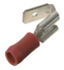
DV18-250P-CY Part Number: **RoHS Compliancy** Compliant Status: DV18-250P-CY replaces DV18-250P-C Note: Part Description: Piggyback Disconnect, vinyl barrel insulated, 22 – 18 AWG, .250 x .032 tab size. Product Type: Disconnects Length (In.): .88 Width (In.): .29 Max. Ins.: .130 Panduit Color Code: Red Tab Size (In.): .250 x .032 CT-100A, CT-260, CT-1550, CT-1551, CT-2500 Tool: Wire Range: 22 - 18 AWG PC Min. Order UOM: Min. Order Qty.: 100 BOM Qty. (# of Pkgs.)
