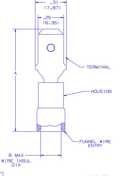
C. STRANDED COPPER WIRE ONLY 2. MATERIAL : A. STAMPING - .031" THK COPPER, NICKEL PLATED B. HOUSING - VINYL
