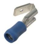
DV14-250P-C Part Number: **RoHS Compliancy** Compliant Status: Part Description: Piggyback Disconnect, vinyl barrel insulated, 16 – 14 AWG, .250 x .032 tab size. Product Type: Disconnects .88 Length (In.): Width (In.): .29 Max. Ins.: .160 Panduit Color Code: Blue Tab Size (In.): .250 x .032 Tool: CT-100A, CT-260, CT-1550, CT-1551, CT-2500 Wire Range: 16 - 14 AWG Min. Order UOM: PC Min. Order Qty.: 100 BOM Qty. (# of Pkgs.)
