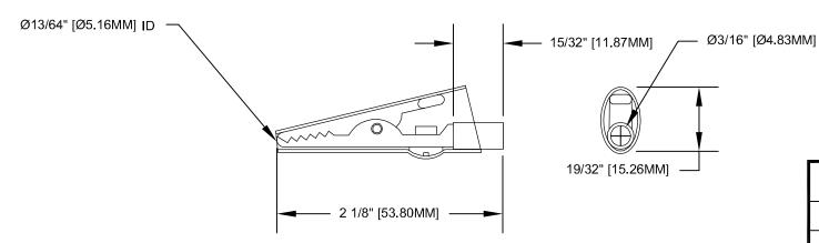
CLIP MATERIAL: STEEL FINISH: NICKEL PLATED INSULATOR MATERIAL: PVC INSULATOR COLORS
