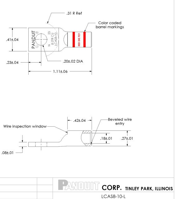
LCAS8-10-L Copper Lug - One-Hole, Short Barrel 10790 **DRAWING NO / CAD FILE** SCALE
