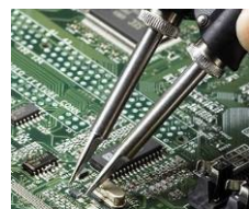
Precision Tweezers handpiece for rework of SMD components with fine dimension to large blade geometries
