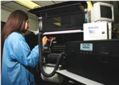
Ideal for cleaning tape and components from feeder trolleys on pick and place machines. An ESD field vacuum is the only way to ensure that these components are not exposed to an ESD event, without removing all of the reels out of a machine prior to cleaning it.
