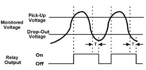
monitored voltage is above the pick-up setting. The relay de-energizes when the monitored voltage is below the drop-out setting for a period longer than the drop-out time delay (T), which is a fixed 500ms for VM Series products. An adjustable time delay on drop-out of 0.5-10 seconds is available (see Page 26).
