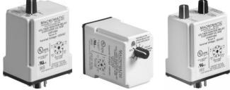
Over/Under Voltage Relays provide protection to equipment where either an over or under voltage condition is potentially damaging. They are designed to operate when the operating voltage reaches a preset value and drop-out when the operating voltage drops to a level below the preset value.
