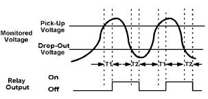
up setting. The relay energizes when the monitored voltage is above the pick-up setting for a period longer than the adjustable pick-up time delay (T1) of 0.1-10 seconds. The relay de-energizes when the monitored voltage is below the drop-out setting for a period longer than the drop-out time delay (T2), which is adjustable from 0.1-10 seconds.
