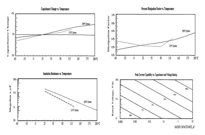
These are typical curves for  $KV^X$  capacitors with mica-paper dielectric. Other dielectric systems are available with improved characteristics. Please contact us for information.
