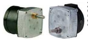
All gears are hobbed to AGMA 7 standards. Pinions are extruded from special steelwith a modified long addendum tooth form to provide higher strength. Pinions are held to the same AGMA 7 quality level as the gears. Both pinion and gear teeth are case hardened for wear resistance and rotate upon hardened and ground steel studs.
