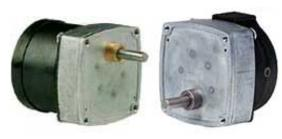
The PA and PB geared motors are the work horses of the Hurst product line. All gears are hobbed to AGMA 7 standards. Pinions are extruded from a special steel with a modified long addendum tooth form to provide higher strength. Both pinions and gear teeth are case hardened and rotate upon hardened and ground steel studs. Synthetic lubrication is used throughout.
