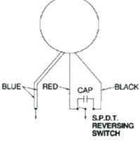
Current applied to the blue and red leads produces CW rotation. Switching the current to the blue and black leads produces CCW rotation. For dual speed versions switching the current produces a change in speed but not in direction of rotation. Direction of rotation must be specified separately.
