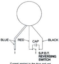
Current applied to the blue and red leads produces CW rotation. Switching the current to the blue and black leads produces CCW rotation.
