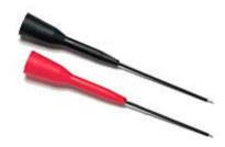
Better than a test probe alone – these two inch long rigid back probe pins easily pass between the weather pack seal and wire. A sharp point ensures good contact to the electrical connector, and the pin's insulation protects it from shorting to other wires.
