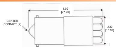
Measurements are typical Dimensions are inches [mm]
