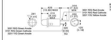
\*\*24 AWG 14" WIRE LEADS - TERMINATION OPTION 007 RED WIRE BLACK WIRE 3001 R/G Red Cathode 3001 R/G Red Anode 3201 Y/G Yellow Cathode 3201 Y/G Yellow Anode 500 .281 [7.41] [3.18]
