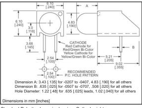
Standard Polarity shown in drawing: Cathode right
