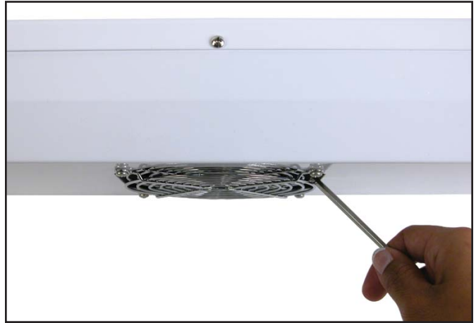
Figure 4. Shorting the ionizer's two fan grills
