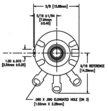
A & B & C DIMENSIONAL VARIABLE. TOLERANCES NOT SPECIFIED  $\pm 1/32$  [0.80mm]
