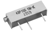
The Model 43 is manufactured to the highest international standards. This product, sealed to  $85^{\circ}$ C for 1 minute (IEC. 68-2-17) has an effective travel of 20 turns nominal and a resistance range of  $10\Omega$  to  $2M\Omega$ .
