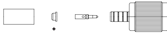
outer ferrule bushing male contact plug body assembly ♦ This part is used only with RG-62 cable
