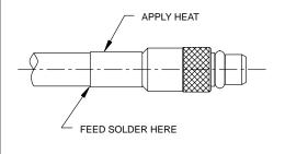
Step 3 Insert contact into body assembly "b" as shown. Holding body and cable firmly, apply heat as shown and feed solder (Sn-60) as indicated. Allow to cool. The dimension from the contact tip to the end of the body should be .006 ±.007.
