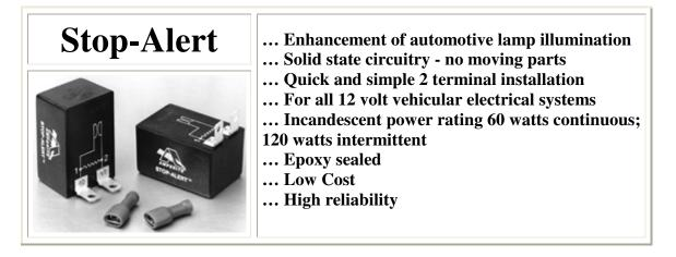
The Amperite Stop-Alert automotive lamp pulsator is a 100% solid state device that is connected in series with one or more automotive lamps. It controls current to the lamps to produce a moderate "pulsating" or "glimmering" effect of the lamp illumination for increased awareness and safety.
