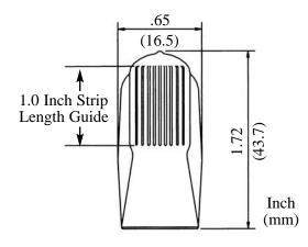
a vinyl insulator. The spring shall have a corrosion resistant coating. (The connector shall be UL Listed and CSA Certified as a pressure cable connector. The connector shall be voltage rated 600 volts maximum, building wire, 1000 volts maximum, signs, fixtures and luminaires. The connector shall have a maximum operating temperature of 105°C.
